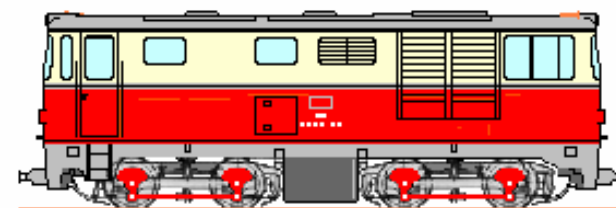
2095.01 to 2095.03 with radiator at No. 1 end
